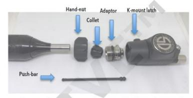
loosen collet hand nut holding the grip then remove adaptor downward from machine head. Note Always Hand tighten collet nut only, do not use tools to tighten.
